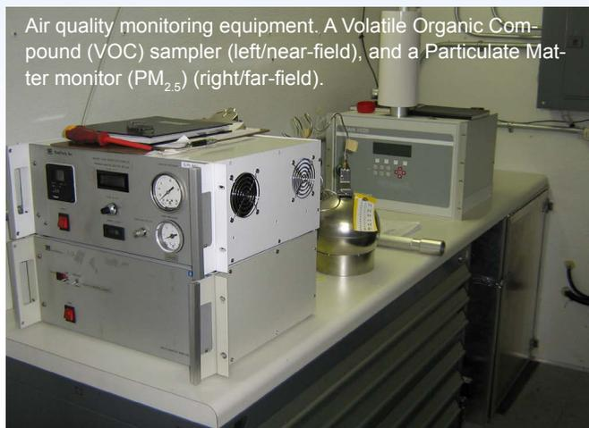
Air quality monitoring equipment. A Volatile Organic Compound (VOC) sampler (left/near-field), and a Particulate Matter monitor (PM<sub>2.5</sub>) (right/far-field).
